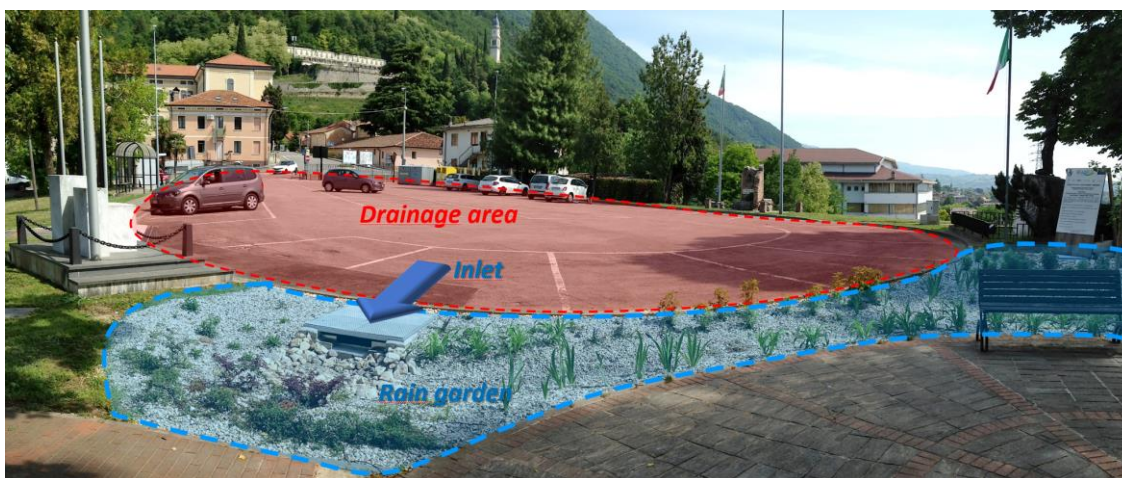
Figure 4.3. Graphic scheme of the functioning of the inlet runoff measurement, with the positioning of the inlet device that collect the runoff from the drainage area (red polygon) measuring the discharges before it enters the intervention (blue polygon).
