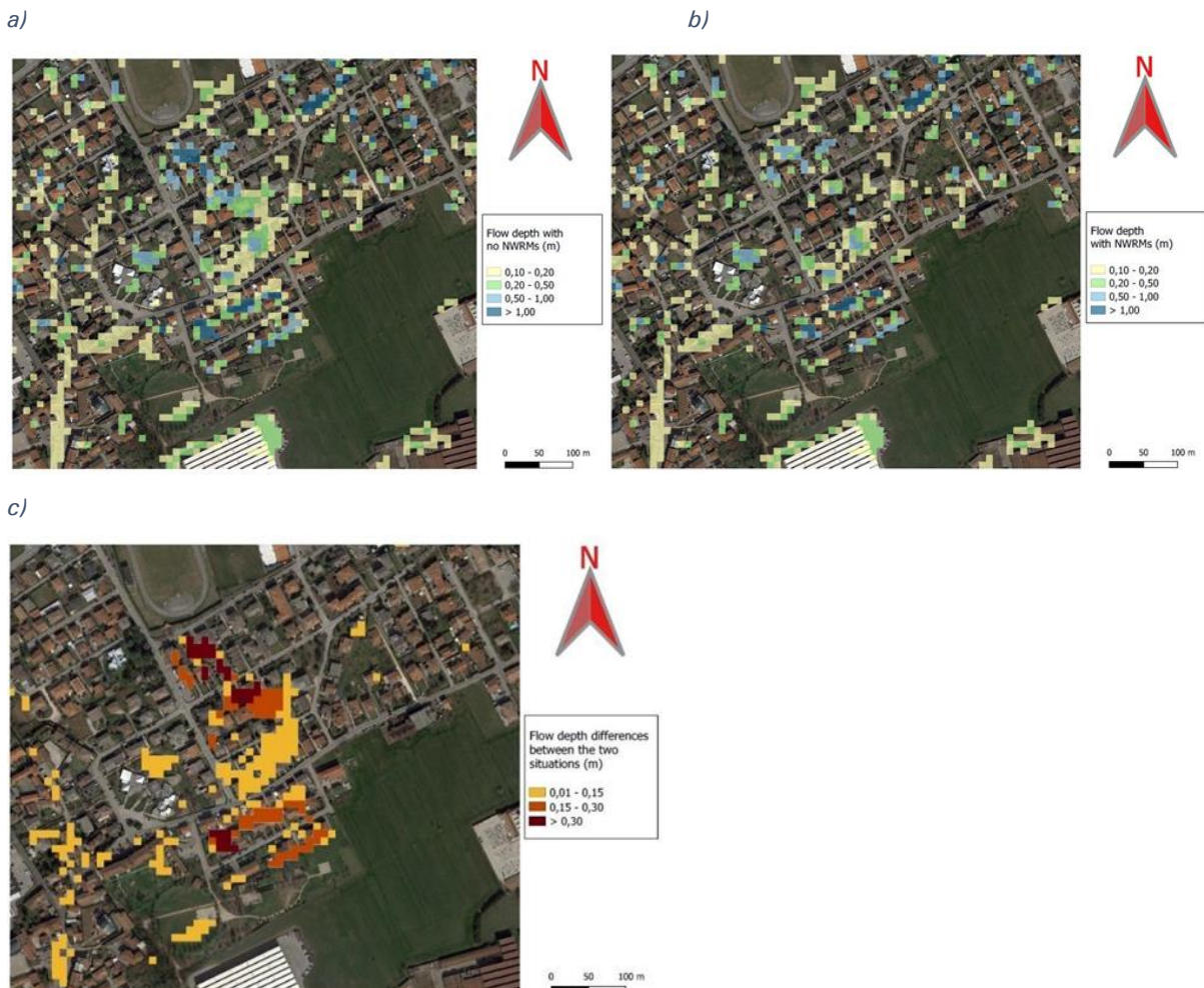
Figure 6: Outcome of the 30-years RP simulation model in an urban area of Marano Vicentino: a) baseline situation (no NWRMs); b) situation with NWRMs; c) difference in the flow depth comparing the two cases.
