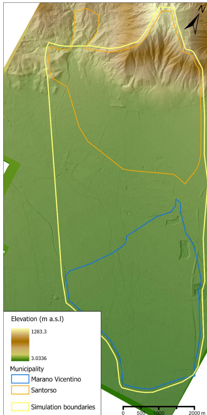
Figure 2. Digital Terrain Model resolution 1m used as base topography for the numerical simulations.
