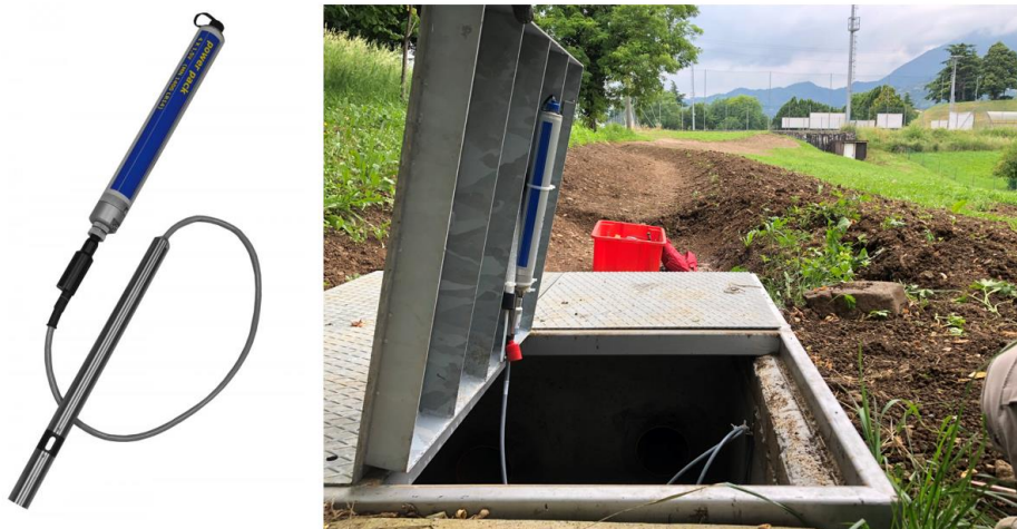
Figure 4.7. The pressure transducer SEBA Dipper-PT used to monitor the flow head over the weir crest (on the left), and a picture of its installation in the Intervention 2 of Action C4 (Grumo hill, Santorso).
