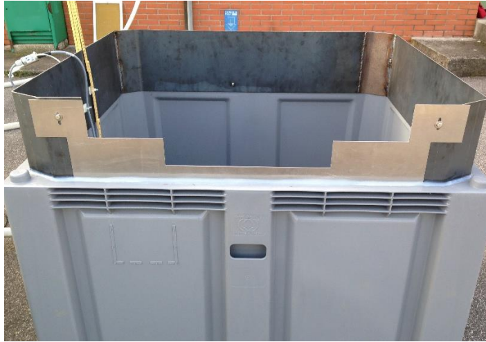
Figure 4.5. Full scale prototype used for the calibration of the CRRSC weir.
